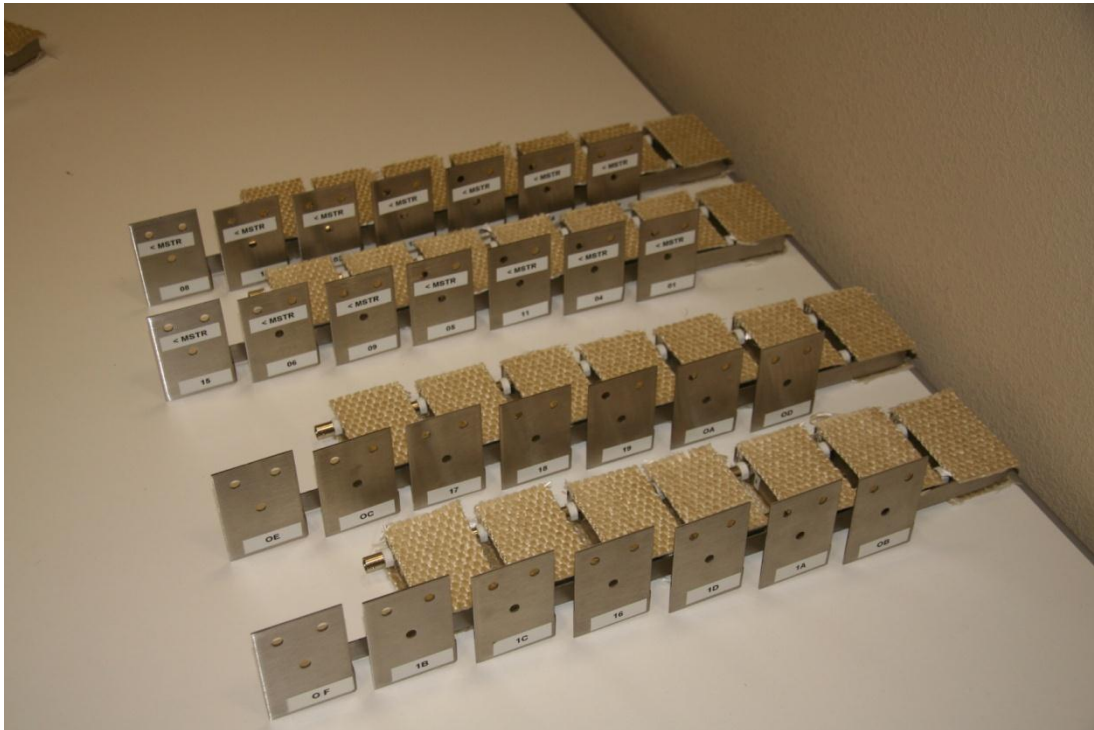
Fig.7. A batch of slaves ready for shipment to the field test. Upper insulation now in place.
