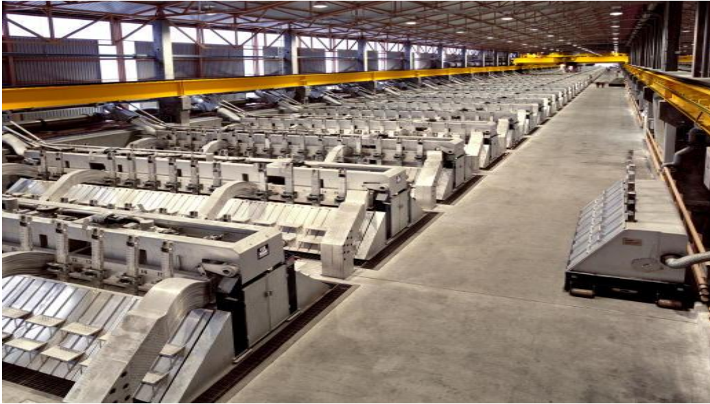
Fig. 4 . A line of cells within an aluminum plant. Approximately 50 cells (“pots”) can be seen but there could be 200 or more cells, connected in series, in this “potline”. Two workers can be seen at the upper right.
