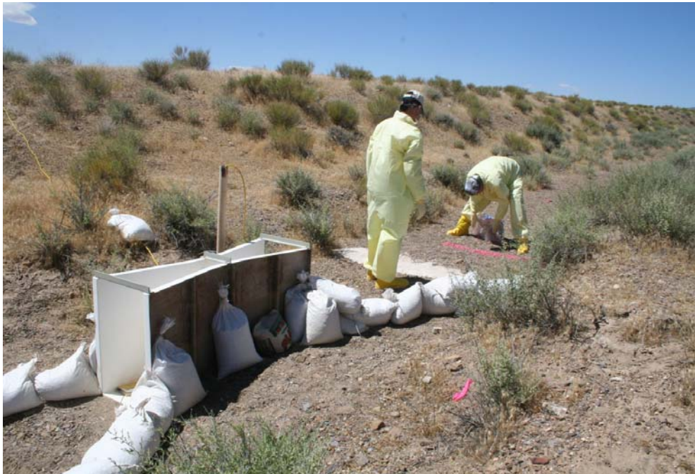
Figure 6. Changes in the downstream edge of the white sand and painted pebble bands will be made to quantify sediment movement during recorded runoff events.
