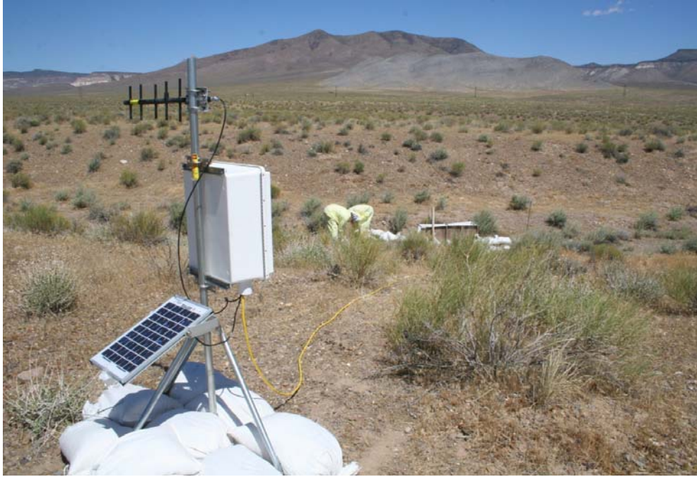
Figure 5. Runoff conditions in the flume are detected by pressure transducer (yellow cable), recorded in the datalogger (white box) and relayed by radio (black antenna) to the meteorological station for transmission to the Western Regional Climate Center via GOES satellite.
