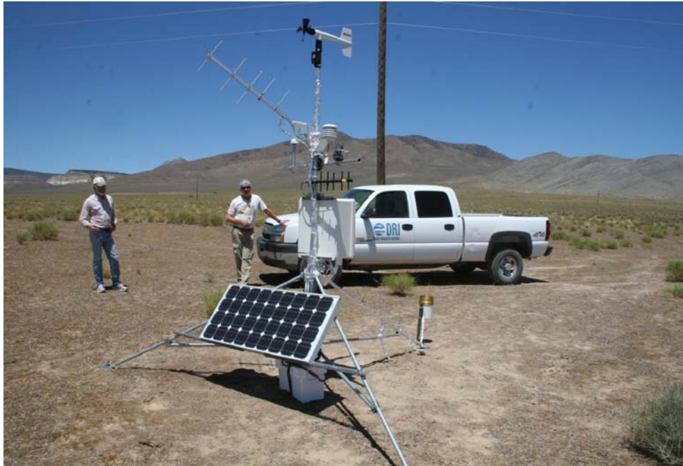
Figure 3. Smoky CA meteorological station was installed to measure precipitation and wind and other climate parameters.
