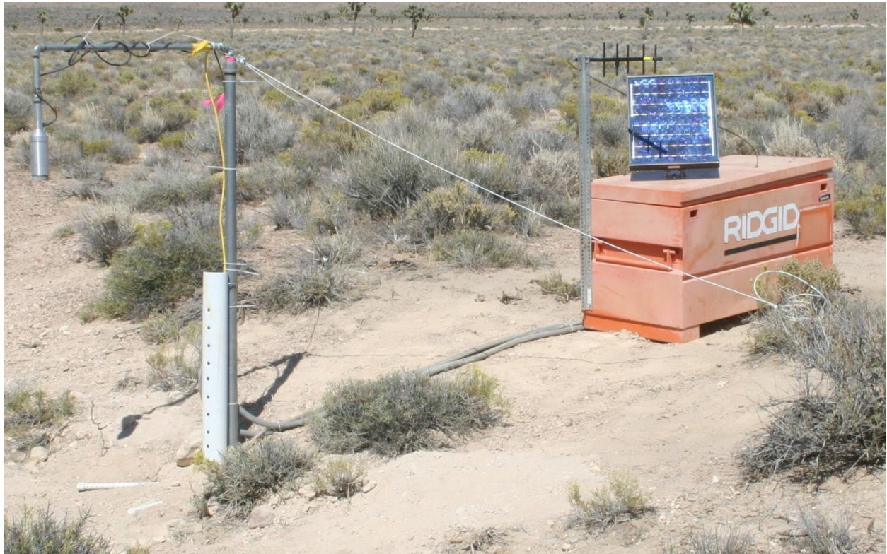
Figure 4. The ISCO sampler (inside the orange job box) is triggered when the pressure transducer (yellow cable in the stilling well) detects runoff. The ultrasonic depth sensor (on the left, hanging from the pole) measures flow depth. Detection of runoff and flow depth data are relayed by radio signal to the south meteorological station and then by GOES satellite to the Western Regional Climate Center.
