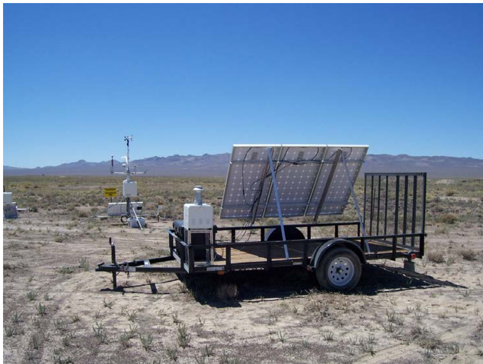
Figure 6. Station 402 solar powered air sampler and portable meteorological station.
