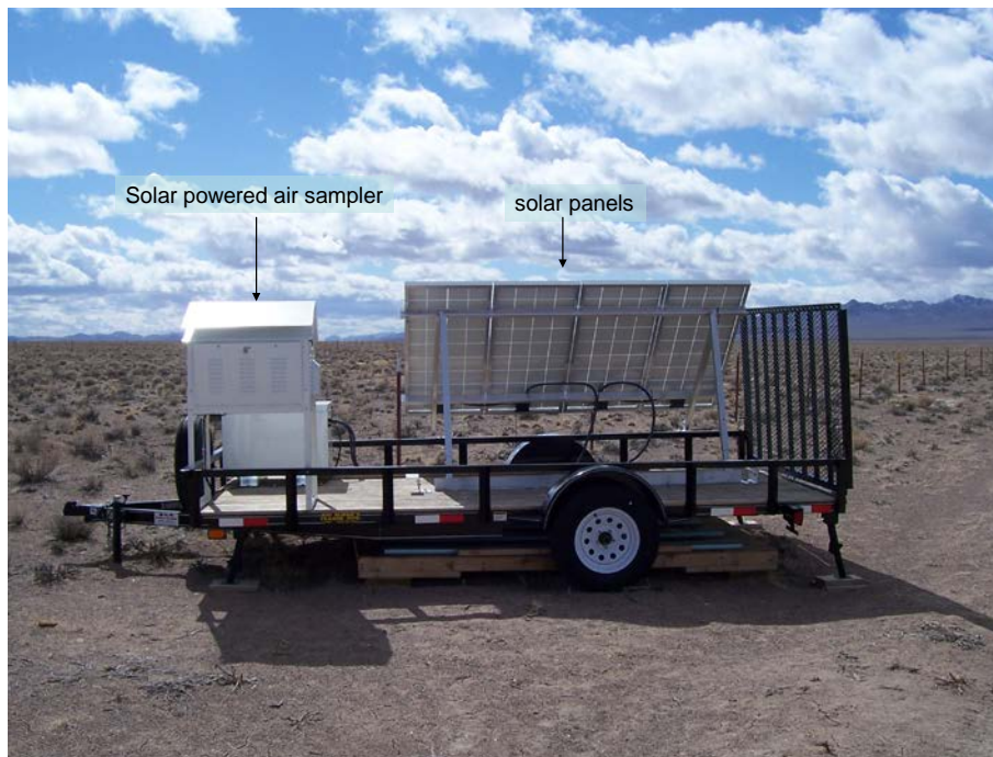
Figure 4. Station 401, solar powered air sampler.
