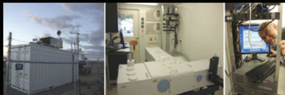
Left: The Remote Sensing Verification Project robotic solar observatory for regional-scale greenhouse gas monitoring deployed at the San Juan substation site near Farmington, NM. Center: In situ laser sensor monitors \text{CO}_2 and \text{CH}_4 continuously from inside the observatory. Right: Instrumentation.
