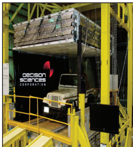
A muon tracking detector invented by LANL scientists and manufactured and sold by Decision Sciences Corporation uses natural cosmic rays to detect smuggled nuclear material in vehicles.
