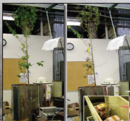
The experimental apparatus, left, shows that water content correlates with the NMR signal (right). During three days of continuously monitoring an aspen tree suffering from drought, researchers saw evidence of changes in water content for day versus night, as well as the overall decline in water content as the tree's health declined.
