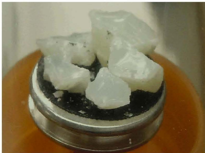
Figure 3. Sn(II)apatite on a Scanning Electron Microscope Mount. (Mount is 1 cm diameter.)
