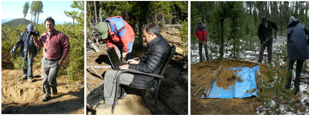
Data quality control: Left to right: Trenton creating an artificial “earthquake”, a computer is connected to the digitizer to see whether the seismometer properly recorded the signals, after confirmation of proper recording, we bury the site and cover the plastic tarp with loose soil.
