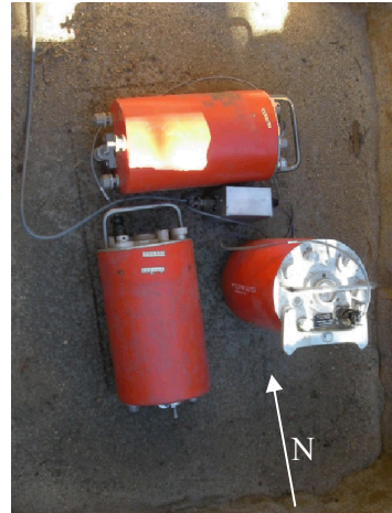
Fig. 2: On the left, schematic showing a three-component GS-13 site (adapted from IRIS website: www.iris.edu .) On the right, a photo from a typical Newberry deployment site of the three single-component seismometers and the resistor box.
