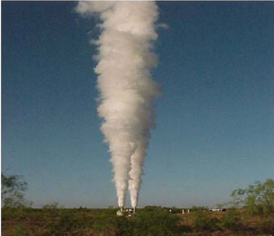
Figure 3. CO 2 release experiment at Dordrecht, Netherlands, by Shell (Kuipjer, 2008). The comparison of the image with Figure 2 can be of help in understanding the evolution of the CO 2 dispersion away from the high-pressure source.
