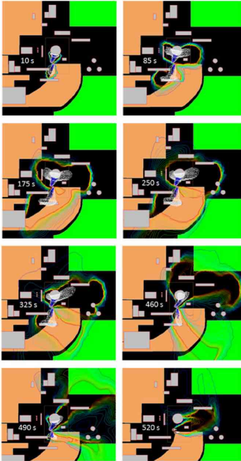
Figure 24. Simulation results showing the CO 2 concentration isopleths (see text) at eight times following the start of the leak for Scenario 4.
