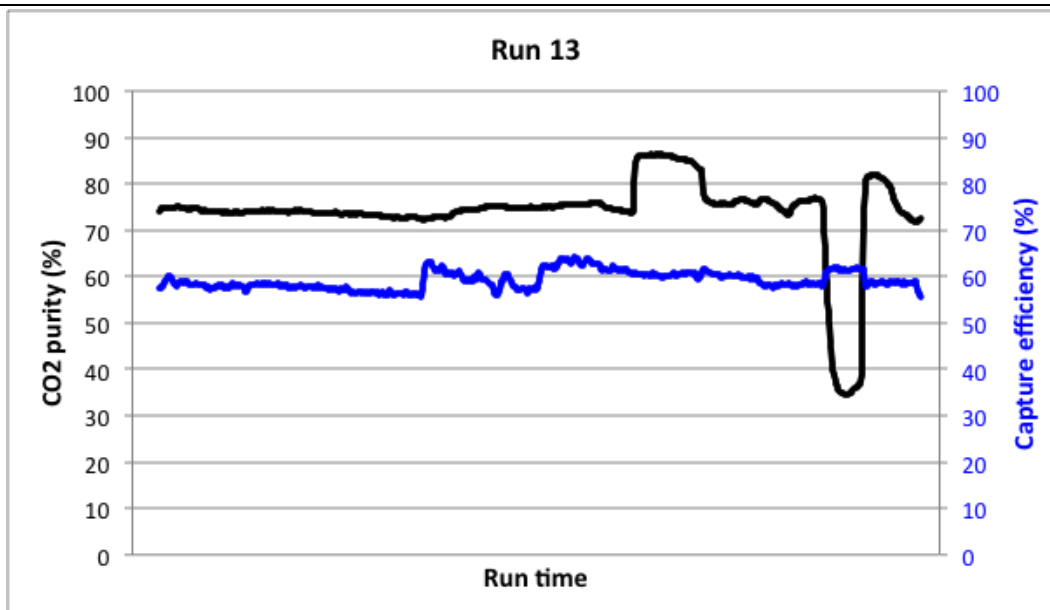
Figure V-22. Results of Run 13 showing stable operation without loss of capture efficiency.
