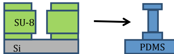
Figure 14: Schematic of a three layer SU8 master to be used as a mold to cast PDMS micro-pillars with stoppers on top. Controlled exposure will be used on layer 2 to create the mold for the pillar.
