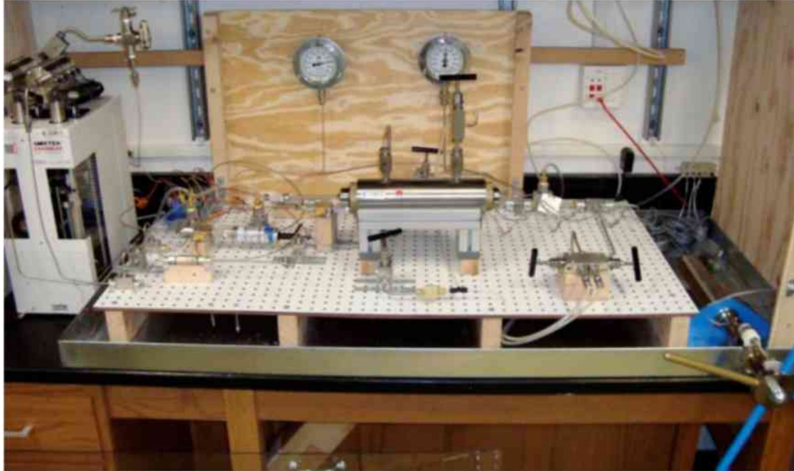
Figure 104: Photograph of hydrostatic permeability system. Quizix pump is on far left, Temco core holder is in the middle, and manual pressure generator is on the far right.
