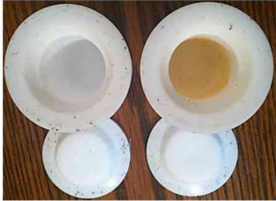
Figure 43. Teflon liner with only CO 2 and H 2 O (to the left) and a Teflon liner containing GHB (Good Harbor Basalt) sample (to the right), showing a precipitation of Fe 2+ mineral phases on the walls of the Teflon liner.
