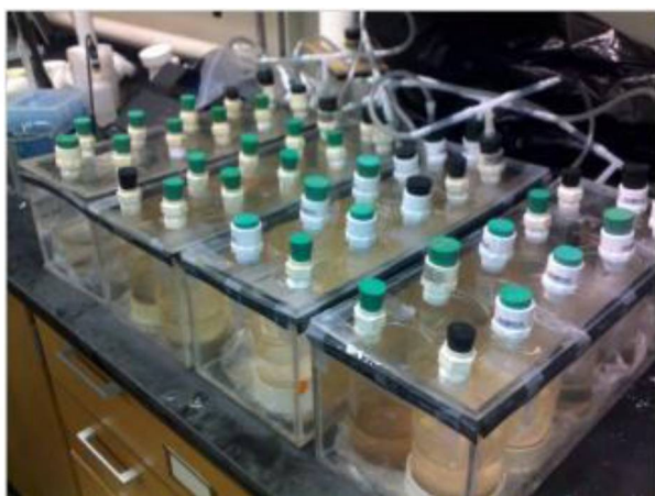
Figure 8. Aquarium tanks used for the continuous flow gas reactors. The solid and liquid reactor components were added in to Nalgene bottles and placed inside the Plexiglas tanks. A \text{CO}_2 concentration of 400 or 1,200 ppm was maintained. Water samples were collected through the top ports for analysis.
