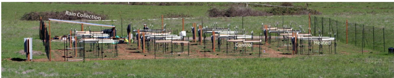
Fig. 1. Example of site infrastructure. At each site, we have 20 plots within a large fenced area. Non-heated plots have ‘dummy’ heaters hung to control for any shading effect from the heat lamps, and there is an on-site rain collection surface for the precipitation treatment.
