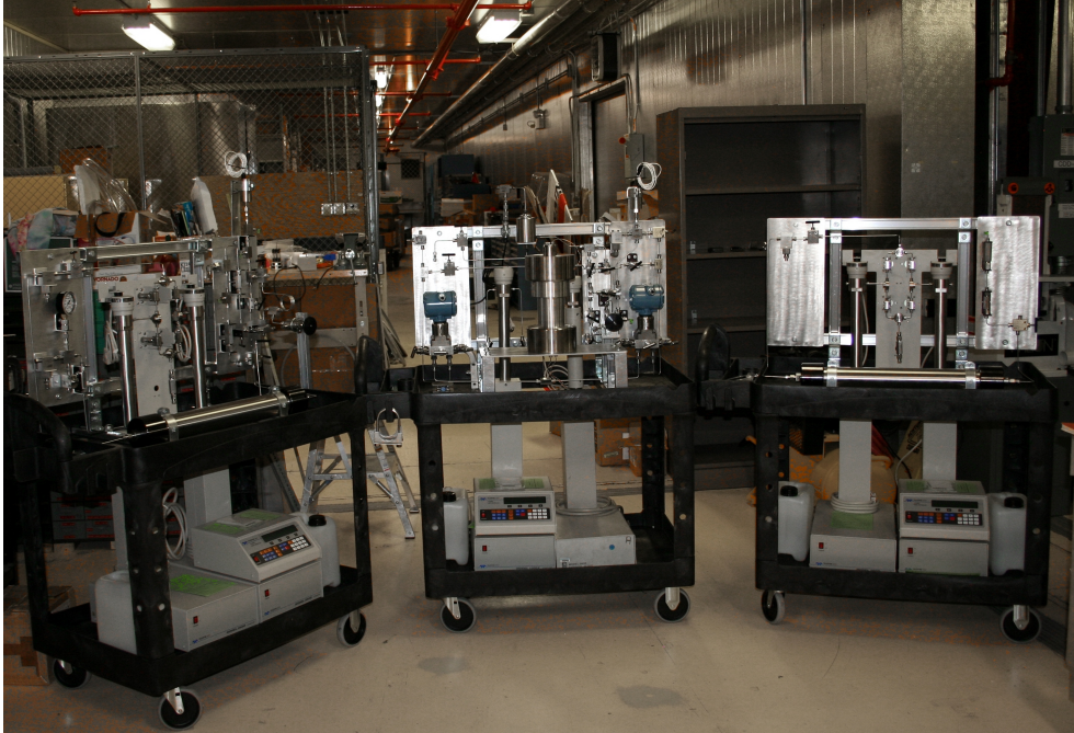
Figure 2. Photograph of the three mobile carts comprising the triaxial coreflood system. The cart on the right deliver brine (cart 1); the cart on the left delivers CO 2 (cart 2); and the cart in the middle contains the coreholder and pumps for delivering the confining fluid and axial load.
