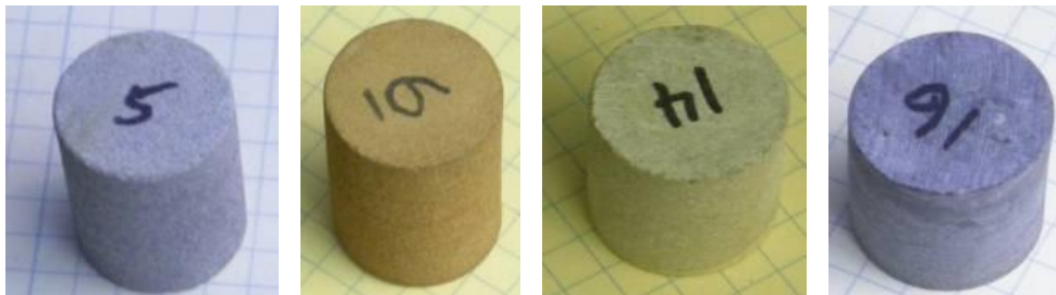
Figure 1-b. Examples of rock core types currently being tested at MTech include: Berea Sandstone (5), Torrey Buff red sandstone (6), Limestone (14), Dolomite (16). Material properties measured include porosity, permeability, pore volume, grain volume, bulk volume, and bulk density. MTech has begun analyzing rock core samples from geologic formations being considered for CO 2 injection. These formations include the Madison Limestone Formation and the Frontier Sandstone formation in the Powder River basin (Wyoming and Montana).
