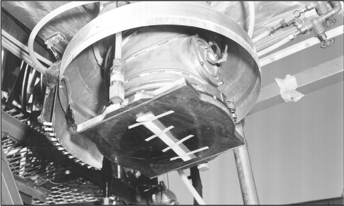
Photo 7. A July 10, 1967 photograph shows the lower portion of the Operation HENRE neutron accelerator mounted in the BREN Tower's payload hoist car elevator. One of the tritium targets is in place at the bottom of the accelerator assembly (Photo 2491-2 on file at NNSA/NSO Nuclear Testing Archive).
