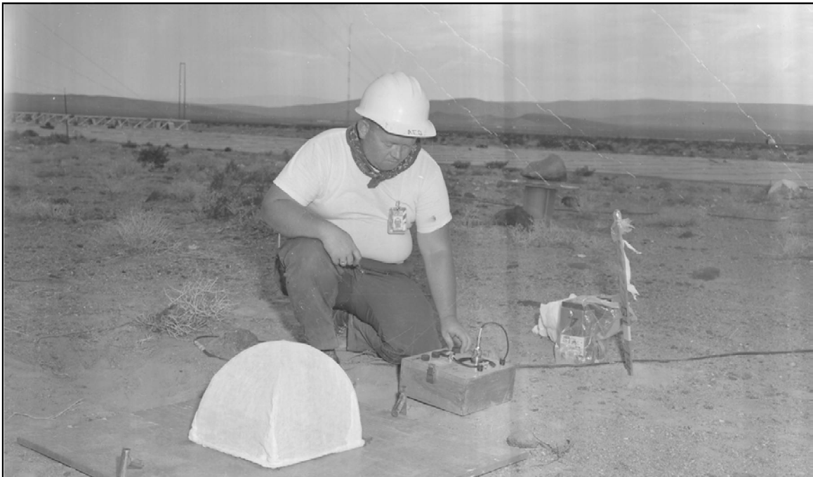
Photo 84. Technician adjusting field instrumentation for the sonic boom experiments. BREN Tower and the double wooden tower from Operation HENRE Program 9 are visible in the distance behind the technician. Photo taken August 25, 1970 (Photo 3219-11 on file at NNSA/NSO Nuclear Testing Archive).
