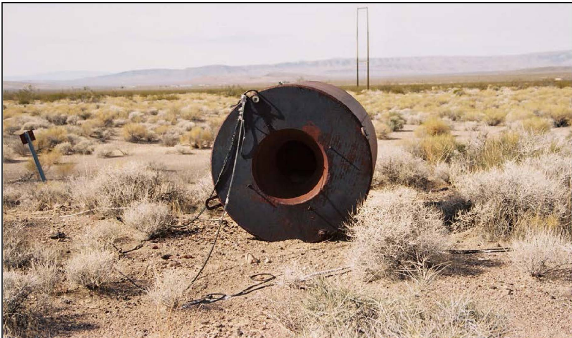
Photo 24. Standard collimator located at 450 ft from BREN Tower. The opening of the collimator is facing southeast. The collimator was used during the Operation HENRE Program 1 dosimetry studies. The Program 9 wooden tower appears in the background. View is to the northwest. Photo taken by DRI on November 1, 2006 (on file at NNSA/NSO Curation Facility).
