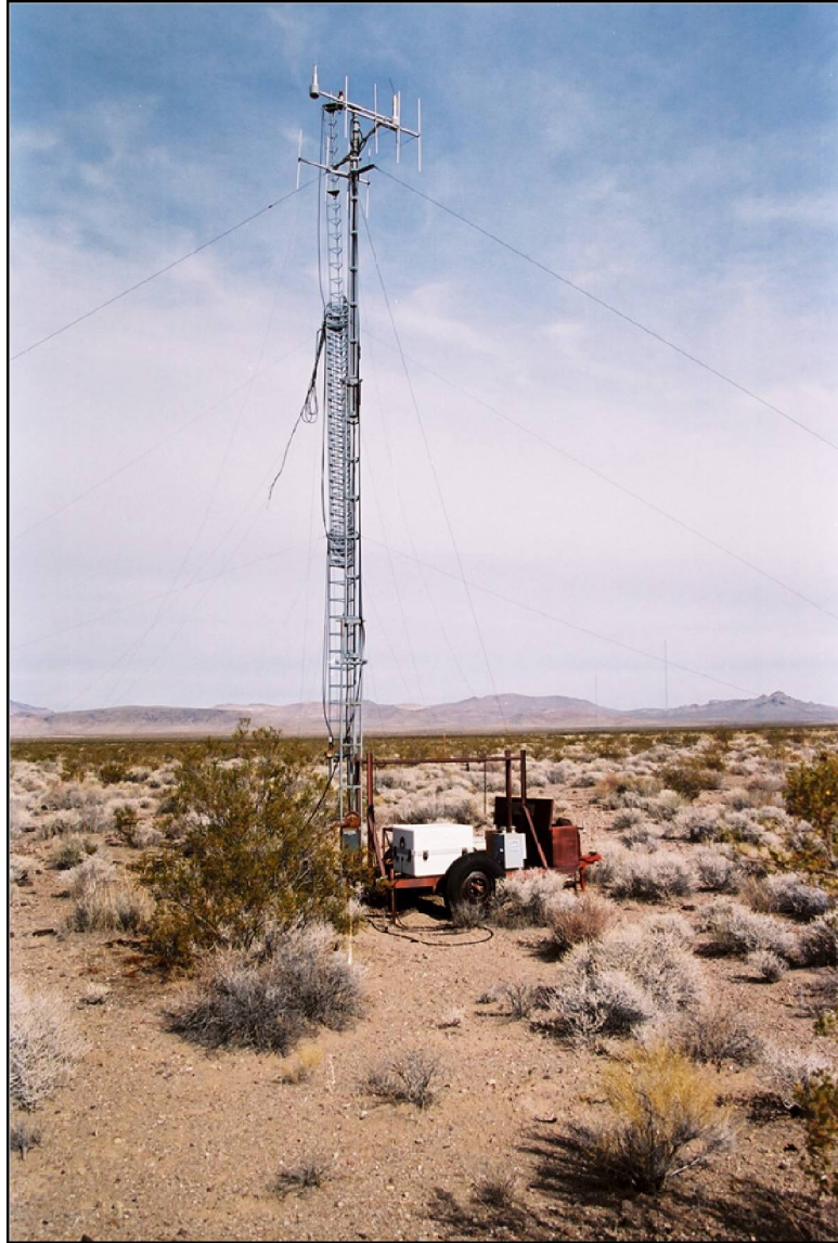
Photo 25. Mobile weather station located 607 ft from BREN Tower. The station consists of an extendable mast with an anemometer, wind direction indicator, and telemetry equipment. The mobile unit positioned alongside the mast included instrumentation to record temperature, barometric pressure, humidity, and precipitation. View to northeast. Photo taken by DRI on November 1, 2006 (on file at NNSA/NSO Curation Facility).
