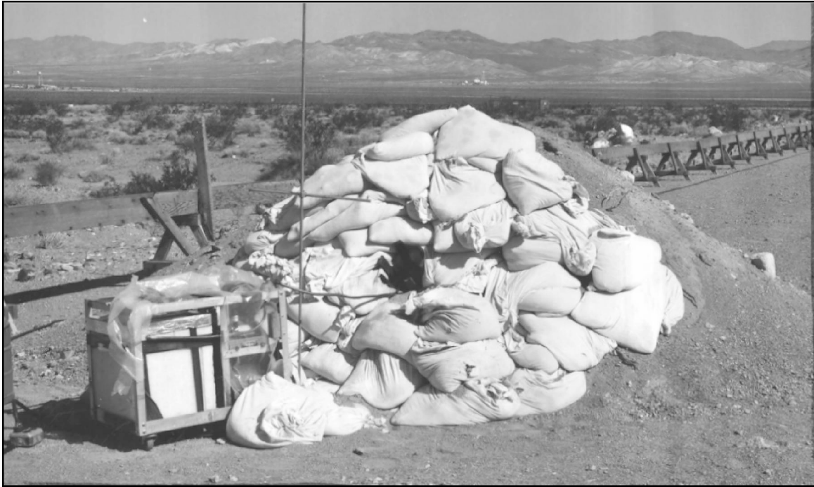
Photo 31. Buried collimator located 1,800 ft from BREN Tower. The surface facing BREN Tower is covered with sandbags, while the collimator body has been covered with earth. August 1967 (Photo 2516-7 on file at NNSA/NSO Nuclear Testing Archive).
