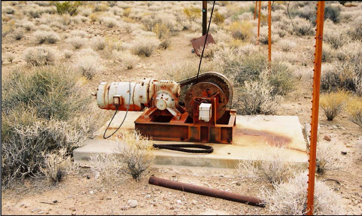
Photo 76. The winch sits adjacent to the wooden tower. It was used to hoist the polyethylene shield and detectors into position for the Program 9 experiments. View is to the north. Photo taken by DRI on November 1, 2006 (on file at NNSA/NSO Curation Facility).
