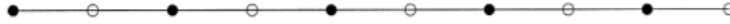
Figure 4.1: Staggered grid for finite difference discretization. Open and closed circles represent displacement and pressure points, respectively.
