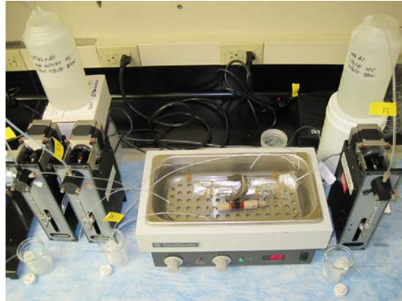
Fig 1.1. Experimental setup for mineral dissolution and secondary precipitation saturated flow-through column experiments under high alkaline condition using PEEK columns, syringe pumps, and water bath (45°C or 89°C).
