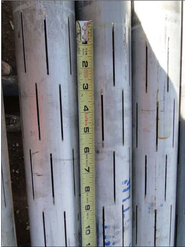
Figure 8-4 Photograph Showing an Example of Slotted Casing
