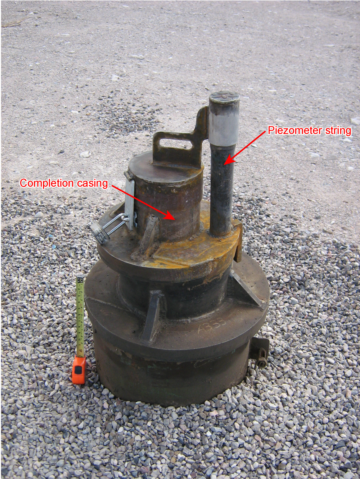
Figure 8-3 Photograph of the Well ER-5-5 Wellhead
