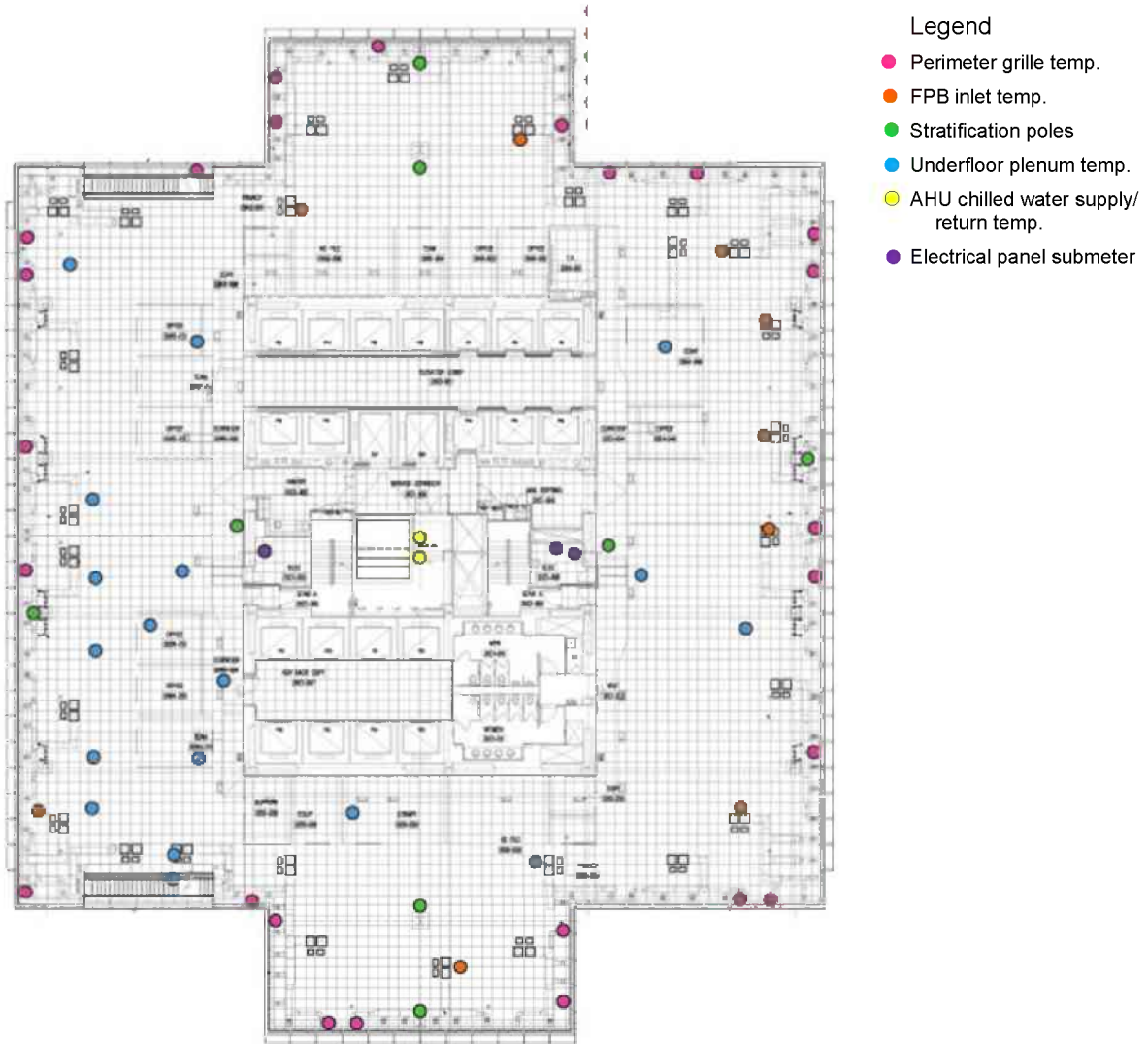
Figure 19. Map of wireless sensors deployed on 20 th floor of the Times Building. Copyright: CBE.
