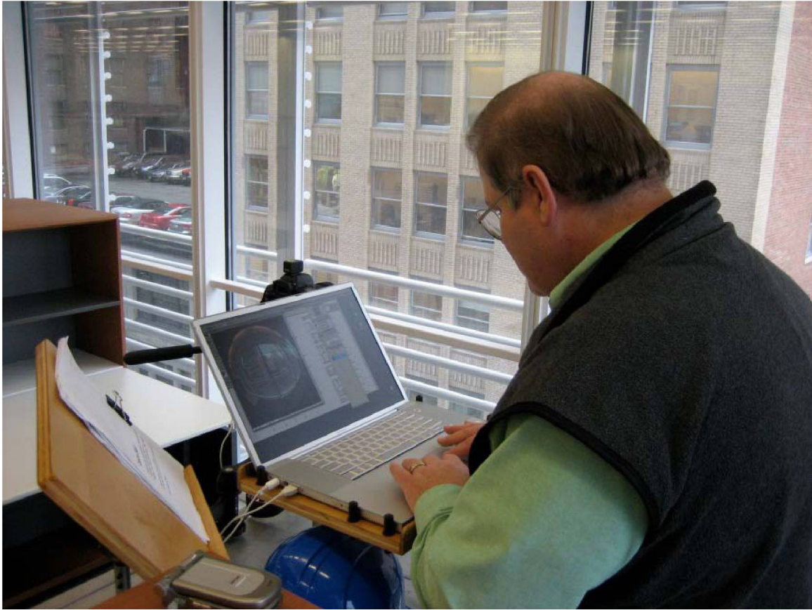
Figure 3. Commissioning cart for the automated shading system being used in the Times Building. Copyright: LBNL.
