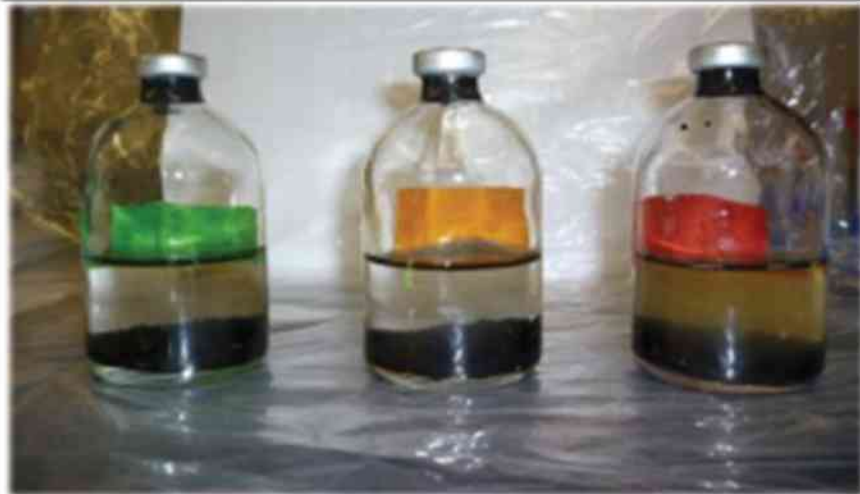
Figure 4. Batch flasks (50 ml serum bottles) containing Powder River coal, simulated coal bed media, and field inoculum.
