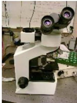
Figure 51. Inspection microscope for the cleaved fiber ends.
