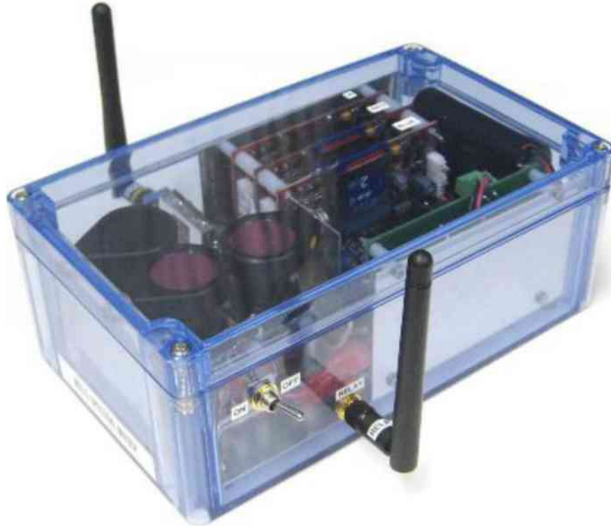
Figure 80. Photograph of the ultra-low-cost spectral imager designed and built at Montana State University for deployment on a tethered balloon.
