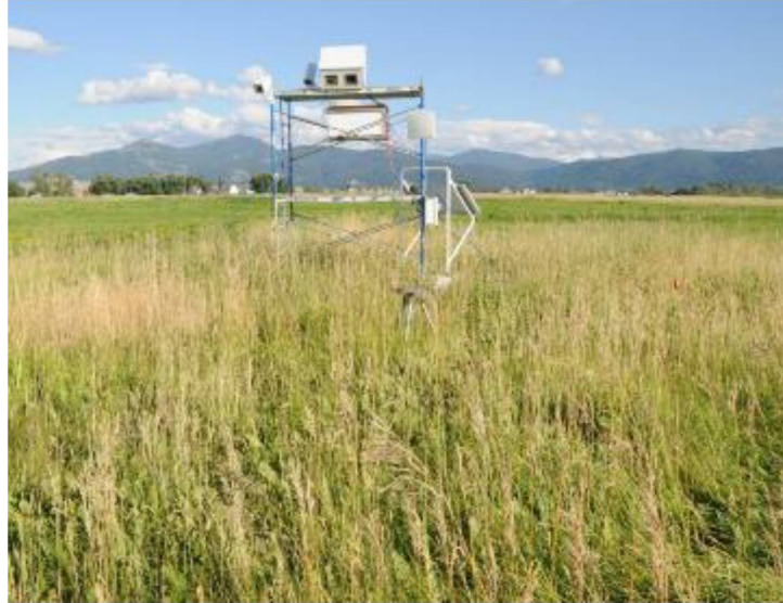
Figure 78. Side-by-side vis/NIR imager and LWIR imager mounted on a scaffold
