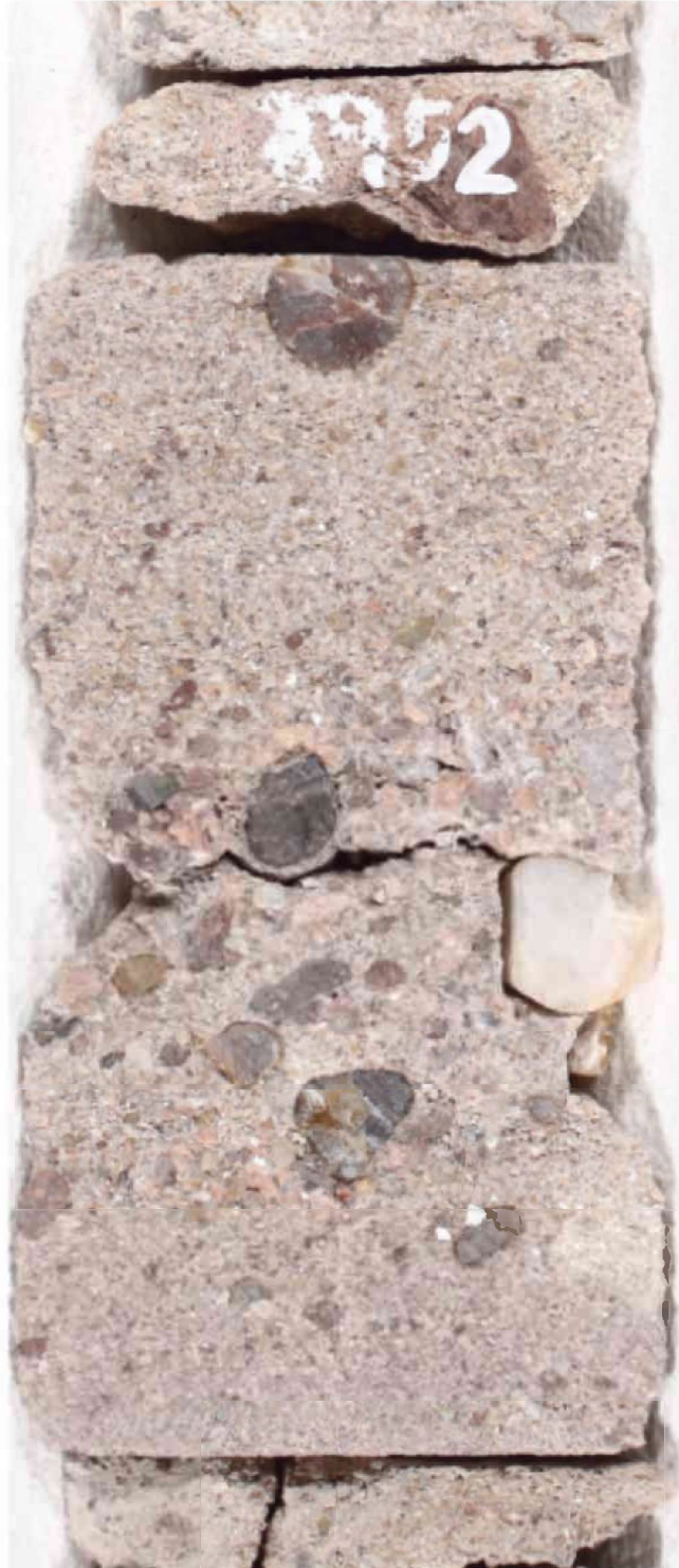
Figure 67 Poorly sorted conglomerate from the lower Mt. Simon Sandstone acquired from Verification Well #2 (measured depth of 2,119 m [6,952 ft]). Pebbles consist of quartz and k-feldspar. The horizontal permeability is 2.22 \times 10^{-9} \text{ cm}^2 (225 md), vertical permeability is 2.37 \times 10^{-9} \text{ cm}^2 (240 md), and porosity is 17%.
