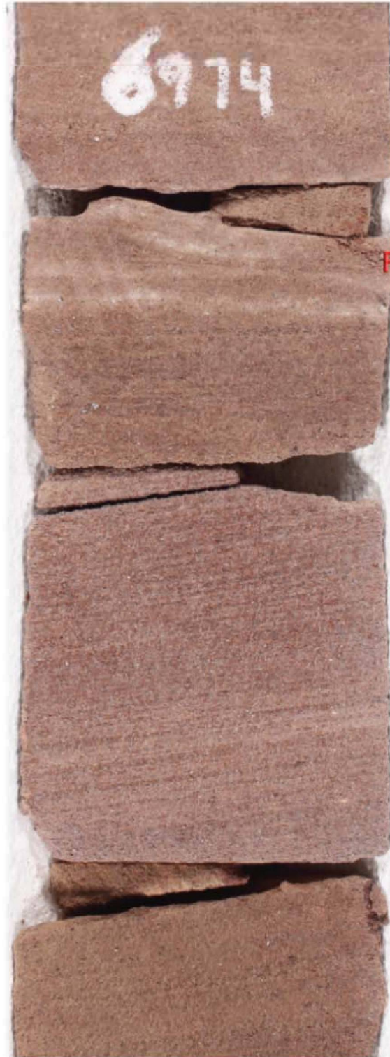
Figure 68 Fine- to medium-grained, cross-bedded eolian sandstone in the lower Mt. Simon from the ADM Verification Well #2 (measured depth of 2,126 m [6,974 ft]). The horizontal permeability is 1.40 \times 10^{-9} \text{ cm}^2 (142 md), vertical permeability is 1.42 \times 10^{-9} \text{ cm}^2 (144 md), and porosity is 22%.
