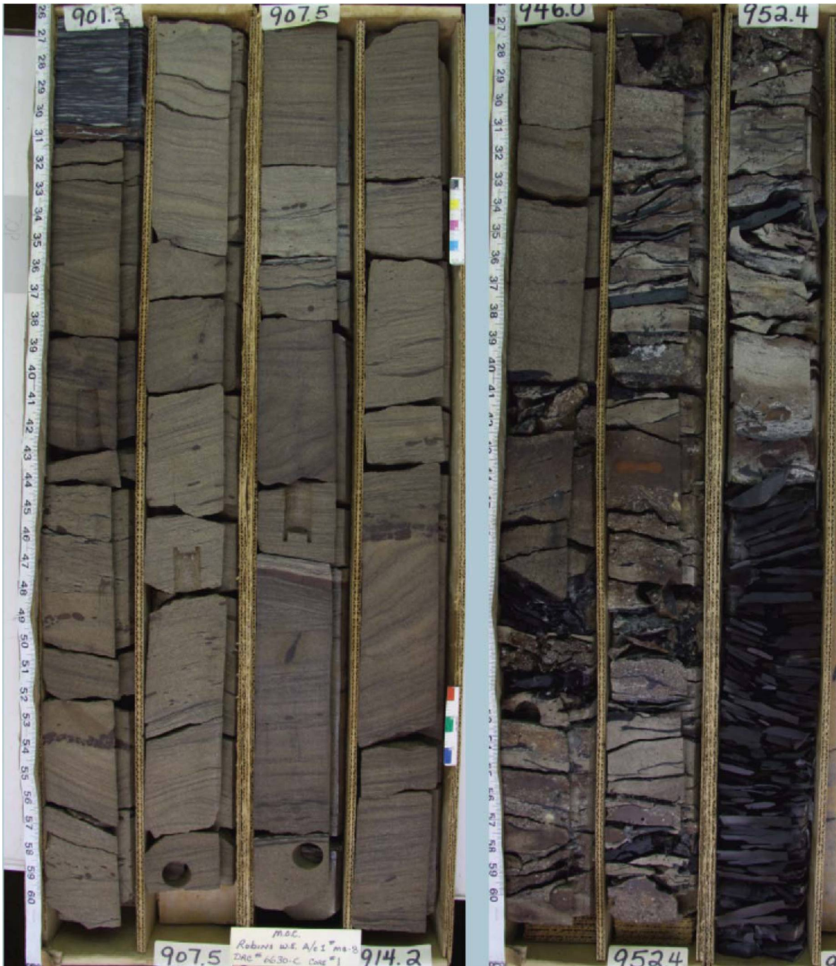
Figure 10 Core example of channel fill Bridgeport B stratigraphic equivalent from the Robbins MG #8 well near the Maraflood pilot in Section 5. Sharp scour contact with coarse rip-up and conglomeratic basal channel lag (approximately 289.56–292 m [950–958 ft]) transitions into very clean tabular cross-bedded sandstone throughout most of the channel facies. Some core shows possible marine indicators in the upper feet of the core (tidal couplets and trace fossils). Channel fill sandstones are generally thicker and have higher permeabilities than their stratigraphic equivalent Bridgeport B deltaic facies sandstones (Figure 11).
