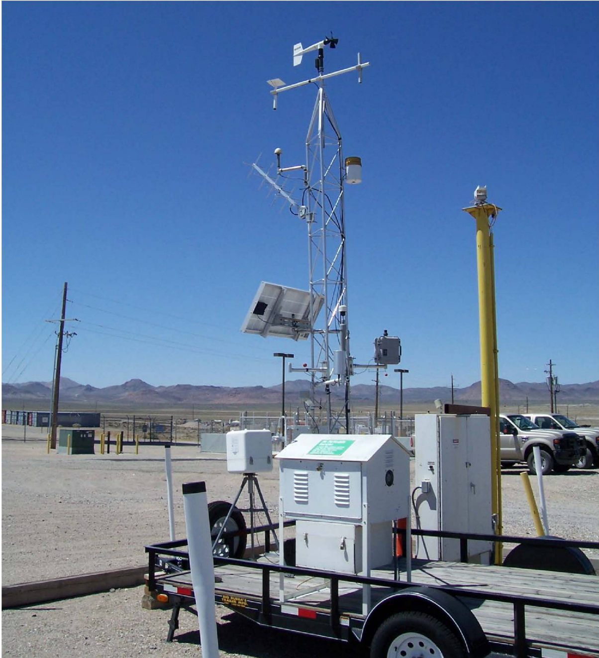
Figure 3. Station 400 is a trailer-mounted radiological and meteorological measurement system located near the Range Operations Center (ROC) at the SNL compound on the TTR.
