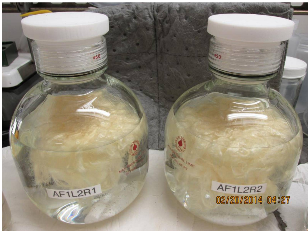
Figure 11. Leno woven adsorbents after amidoximation reaction.
