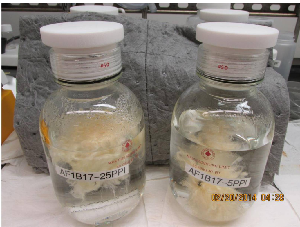
Figure 12. Braided adsorbents after amidoximation reaction.
