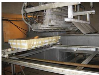
Figure 10. Electron beam set-up used for irradiating braids and leno woven fabrics.
