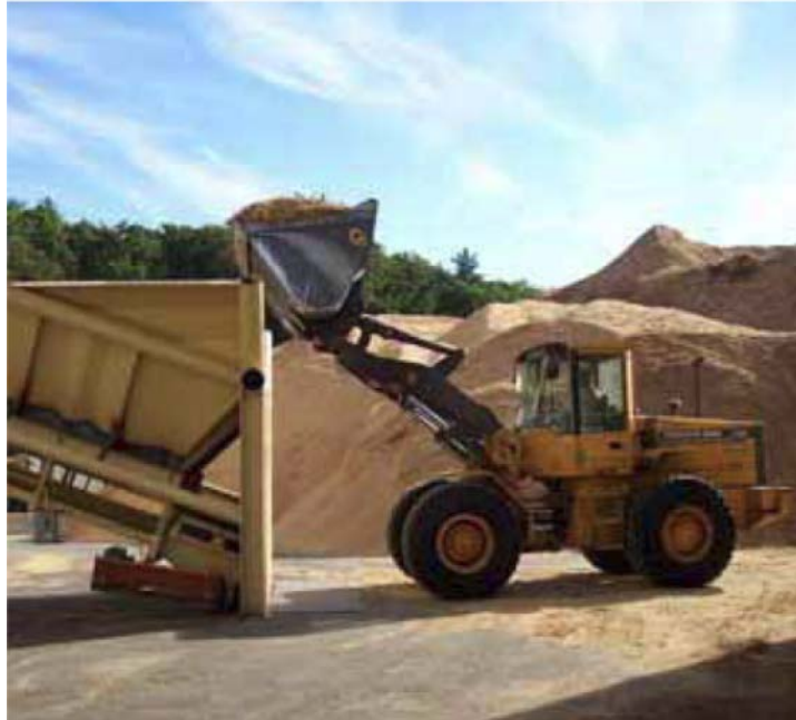
Figure 15. Front end loader transferring materials
