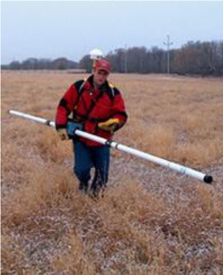
Figure 1 Photo of the EM31-MK2 in Use (Geonics, 2012)
