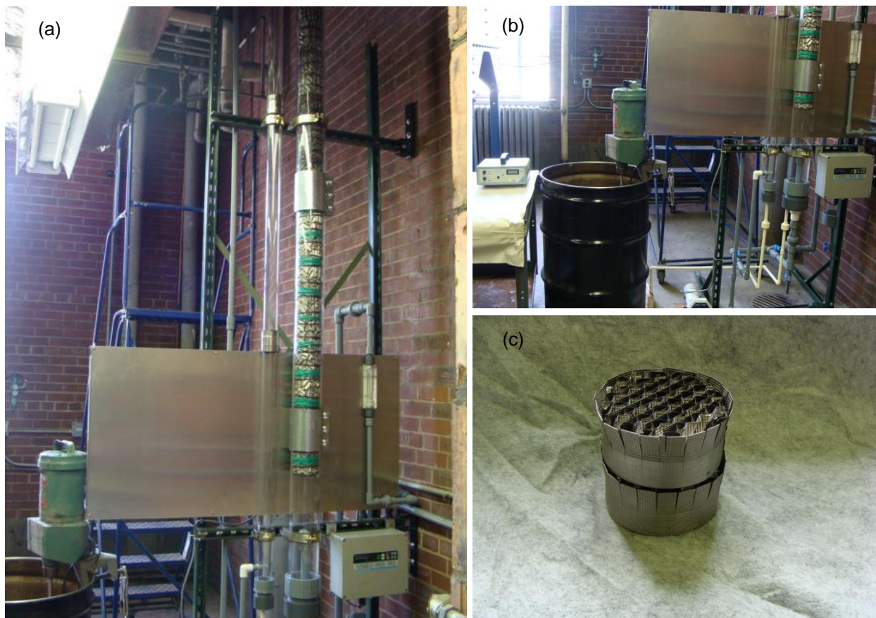
Figure 2B-2. Photographs of the bench-scale packed-bed absorption column: (a) overview of the column setup; (b) solution supply tank with stirrer and temperature-controlled heater; (3) packing unit (10 cm in diameter by 10 cm high).
