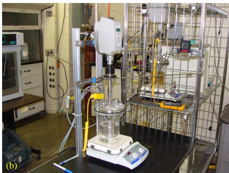
Figure 2A-1. (a) Schematic and (b) Photograph of a STR experimental system. (PrC: pressure controller, PG: pressure gauge, TC: thermocouple, DAQ: data acquisition)
