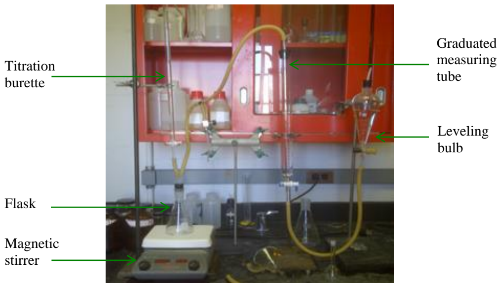
Figure 2B-3. Photograph of the Chittick apparatus used for the CO 2 loading measurement.
