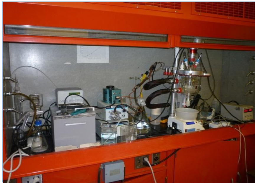
Figure 3A-1. Schematic and photograph of a continuous MSMPR reactor setup.
