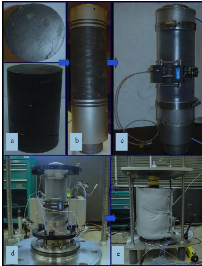
Figure 4: Triaxial Cell Setup used for Measurement of Flow and Ultrasonic Velocities
