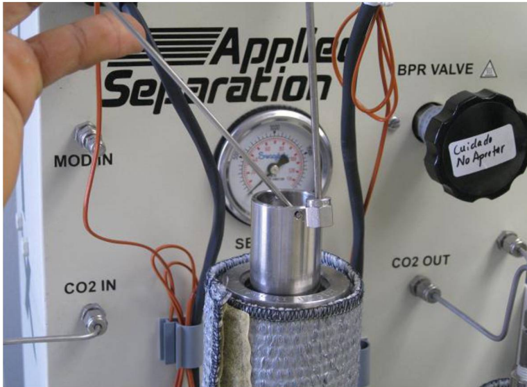
Fig. 5. Introduction of the Basket with the Cylindrical Template Inside the Supercritical Dryer.
