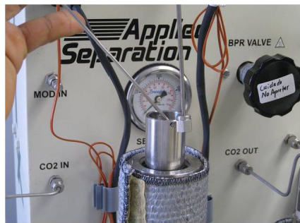
Fig. 2. Introduction of the Basket with the Cylindrical Template Inside the Supercritical Dryer.
