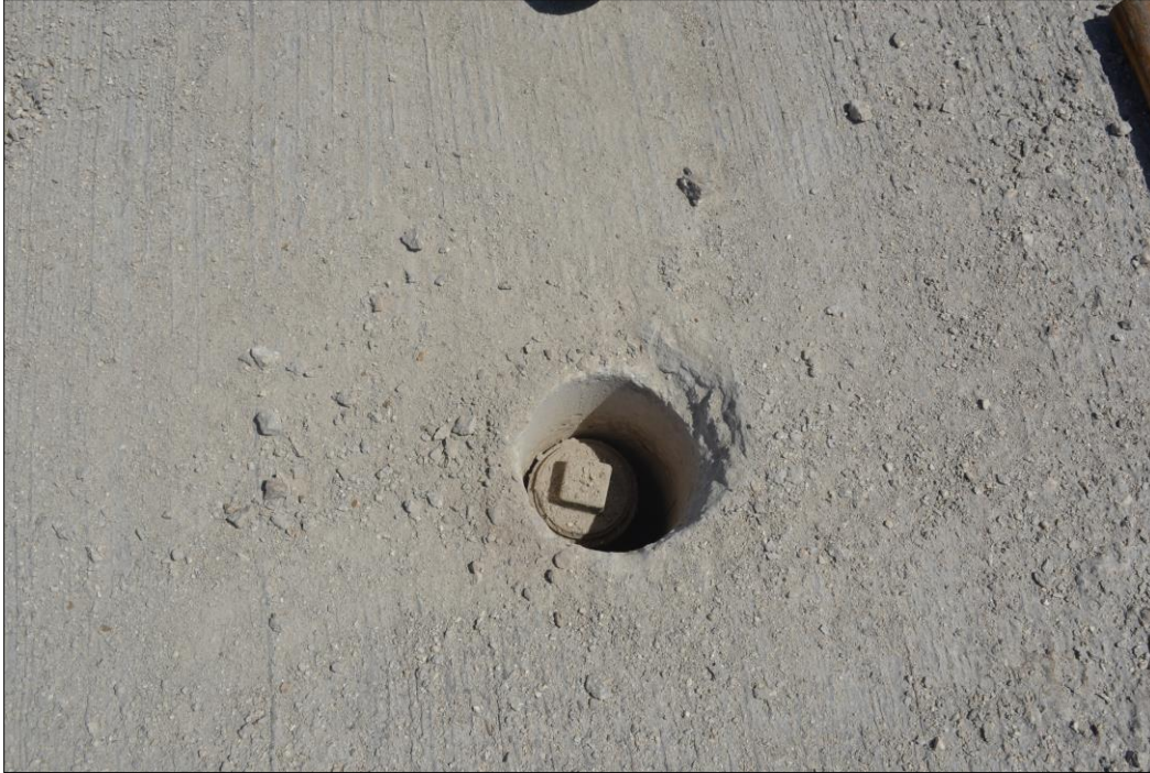
Fig. 10. Recovered borehole (CD-17), originally established in support of a NAS investigation conducted during March 1980 (Visual Survey, May 2013).
