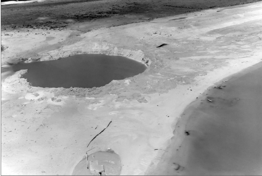
Fig 1. Post-shot view of the nuclear test crater formed by the 18-kt Cactus test conducted on the north end of Runit Island, Enewetak Atoll.
