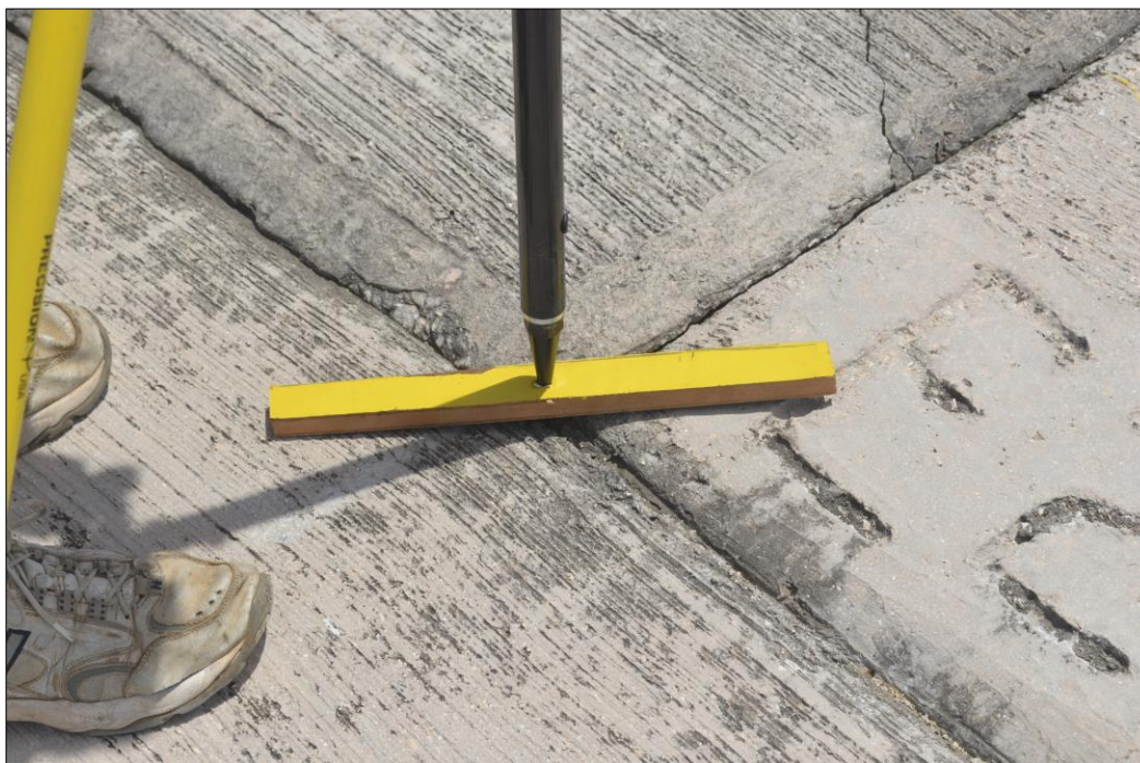
Fig. 9. Photo showing the method for positioning the prism pole while surveying panel corners (RTK-GNSS Survey, November 2013) [the end of the pole is seated inside a wooden paddle containing a beveled out hole].
