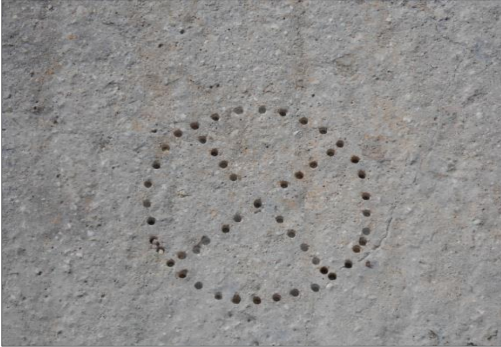
Fig. 7. RTK-GNSS benchmark site placed on a pre-existing concrete block located about 100 meters from Runit Dome (N 11° 33' 8.75464"; E 162° 20' 45.09224") [the survey position is represented by the center most hole drilled in the concrete].
