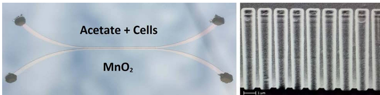
Figure 3: A picture of the microfluidic reactor (left) showing experimental conditions, and an SEM image of the physical barrier (right) that separates the center region where the two channels meet.
