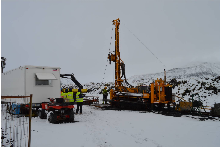
Figure 9. Wireline diamond drilling rig at the CarbFix injection site in October 2014. Photo: M. Stute.
