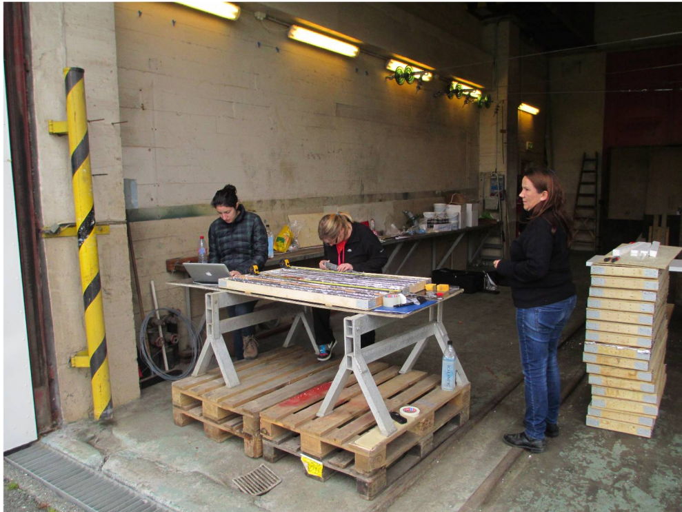
Figure 11. Detailed core description and collection of sub-core samples for XRD, thin section and isotopic analyses. Photo: J. Matter.
