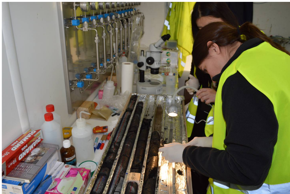
Figure 10. Core description and collection of sub-core samples for microbiological and mineralogical analyses at the CarbFix injection site. Photo: J. Matter.
