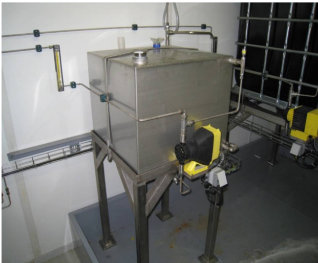
Figure 5. \text{H}^{14}\text{CO}_3 -solution storage tank (100 L) with micro-metering pump attached at the front. Amount of tracer solution injected was regulated by the injection system control system and depended on the actual \text{CO}_2/\text{H}_2\text{O} injection ratio in the injection borehole. Photo: J. Matter
