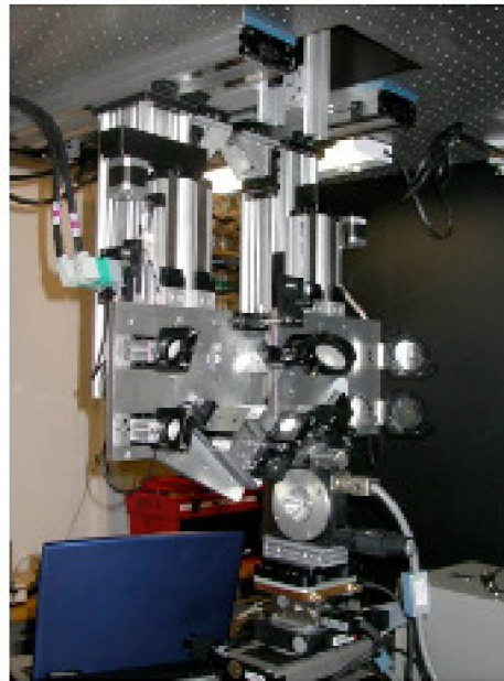
Fig. 4: Schematic (left) and photograph of the Brillouin scattering system at beamline 13BM-D (GSECARS, APS).
