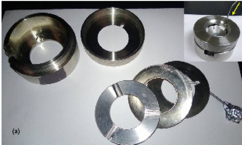
Figure 8: Photo of gas membrane, and membrane “caps” (containers) produced at UIUC for fine control of pressure with conventional diamond cells. The assembled adaptors with a DAC ready for use is shown at the top right.
