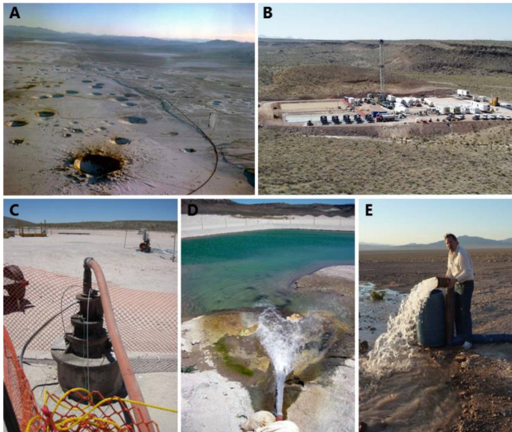
Fig. 2. Examples of sampling sites. A) Yucca Flat from the air (NTS Photo Library, http://www.nv.doe.gov/library/photos/nts.aspx ); B) ER-EC-13 being drilled, from Bill Wilborn, publicly-released 2011 Devils Hole Workshop Talk; C) ER-EC-13 during hydrologic pumping test; D) water discharge at end of pumping test; and E) Amargosa Valley reference well, BLM-1, during pumping test, Jamie Walker (NWRPO) shown. All images from published sources (upper) or cleared for this work (lower).
