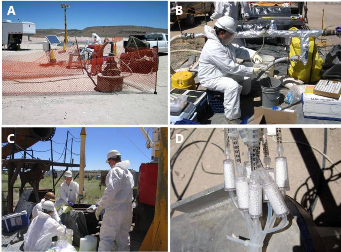
Fig. 3. Microbiological sampling. A) Non-radioactive Pahute Mesa well being sampled; B) PI Moser sampling U19ad PS#1A (Chancellor), a well both high in radioactivity and temperature; C) U12n.Vent.10 being sampled through mountain-top vent hole via improvised bailer; D) Sterivex filter array during pumped sampling of a well on Pahute Mesa, used for DNA-based analyses. Note: dissolved gases accumulating as bubbles (All photos cleared).
