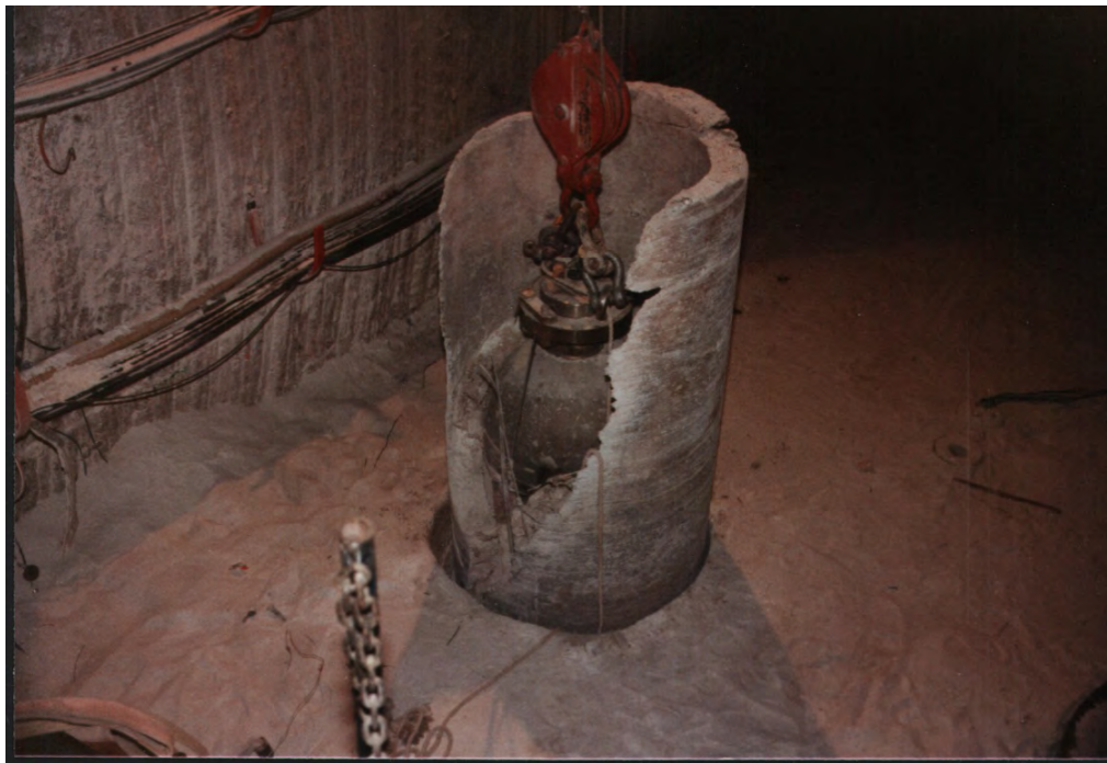
Figure 6: Heater from borehole BO45 showing porosity reduction as a likely result of heat pipe activity (Krumhansl et al., 1991). From Brady et al. (2013).
