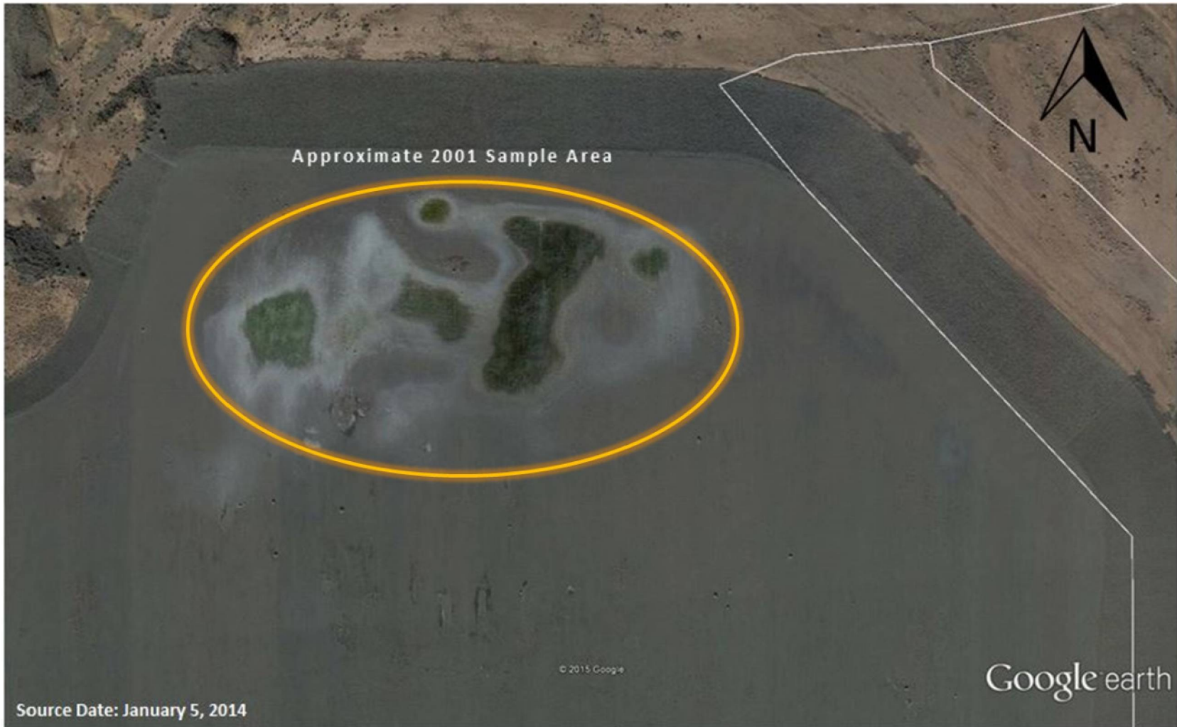
Figure 2. Bluewater, New Mexico, Disposal Cell Evaporite Deposits
