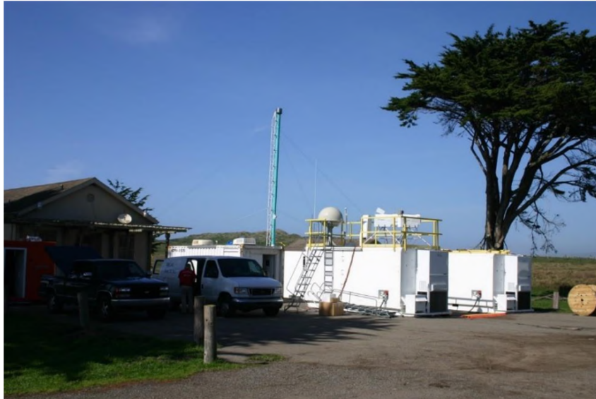
Figure 1. The AMF1 in its initial deployment at Pt. Reyes, California in 2005. It was housed in four shipping containers and included 30 instruments.
