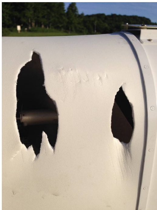
Figure 4. Bear damage to MWR2C radome.
