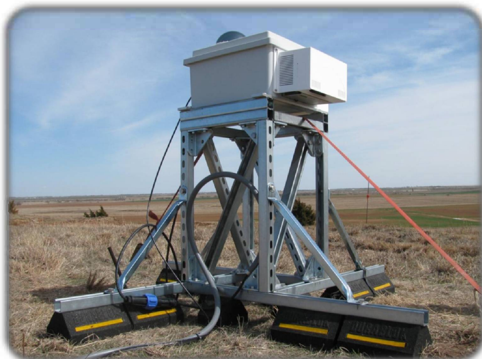
Figure 1. A UCSD Sky Imager deployed in the field.
