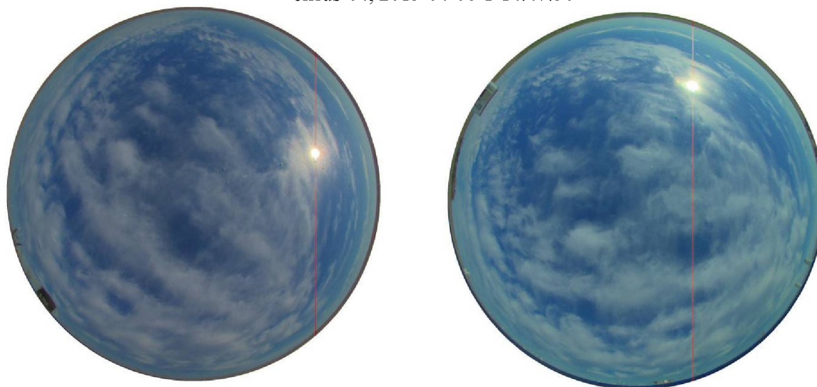
Figure 6. Image pairs for which a dense estimation of cloud position was performed. Images on the left are from USI 1.7 (note Farmer Bobbit's roundtop barn), and images on the right are from USI 1.8. All images are color corrected HDR with a logarithmic intensity rescaling (similar to gamma correction). ( continued )
