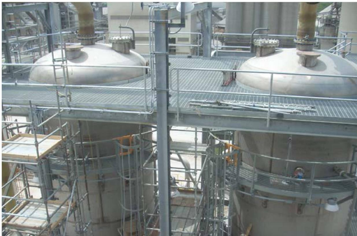
Figure 11 Sodium Bicarbonate Bubble Columns
