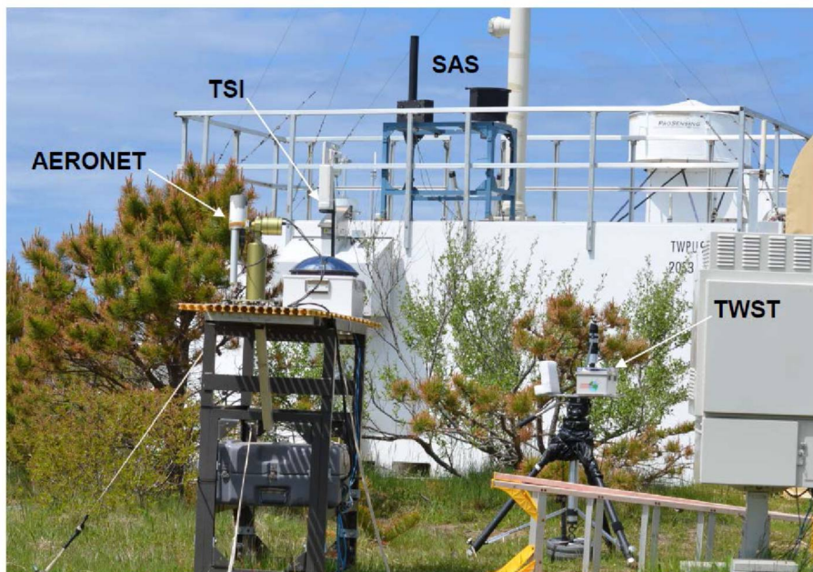
Figure 7. Location of TWST, AERONET, TSI and SAS at ARM Highlands site Cape Cod, MA. All sensors were heavily anchored in place to survive the high wind conditions.
