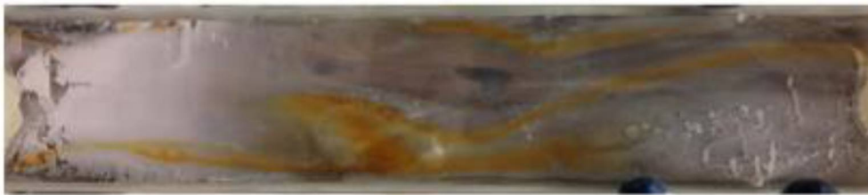
Fig. 34 – Hydrochloric acid (pH 2.29) preflushed cement core (6FP-27) after 24 hours polymer shut-in. White calcium precipitation with rust-colored precipitate (Patterson 2014).
