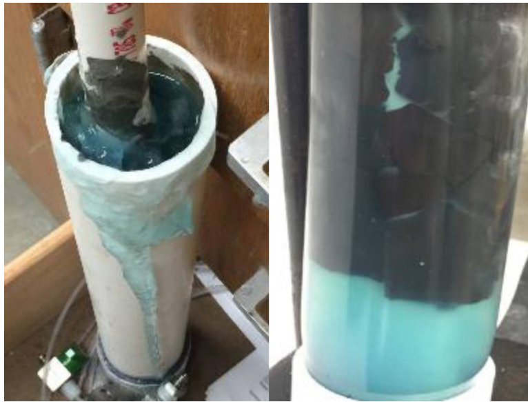
Fig. 37 - Experiment PVC-1 (left) and TYG-1 (right) successfully held 15 psi/ft constant pressure for one week. During pressure breakthrough test, PVC-1 had the maximum breakthrough at 63 psi/ft and TYG-1 (right) had the maximum breakthrough at 25.6 psi/ft.
