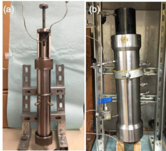
Fig. 16 – Specifications of the 12"-long steel coreholders manufactured by Pheonix Instruments (a) 1" diameter Hassler coreholder (working pressure: 1,250 psi), and (b) 2" diameter Hassler coreholder (working pressure: 5,000 psi).
