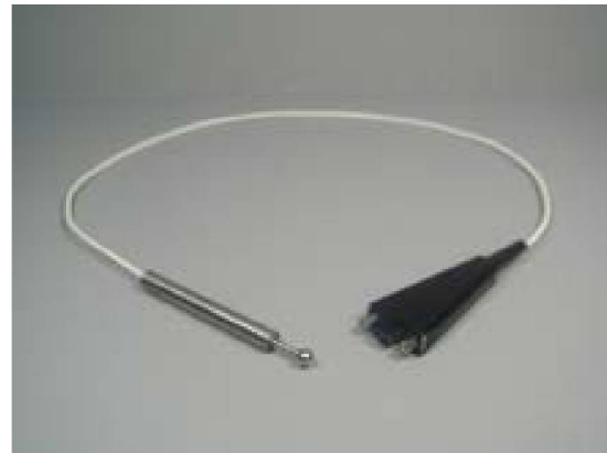
Figure 4.1-1. DVRT (cylinder on left) with signal conditioner (black triangle). DVRT consists of an outer coil in a cylindrical housing with an inner core tipped with a ball. The inner core slides on a bearing at the end of the cylindrical housing. From: http://www.microstrain.com/displacement/sg-dvrt
