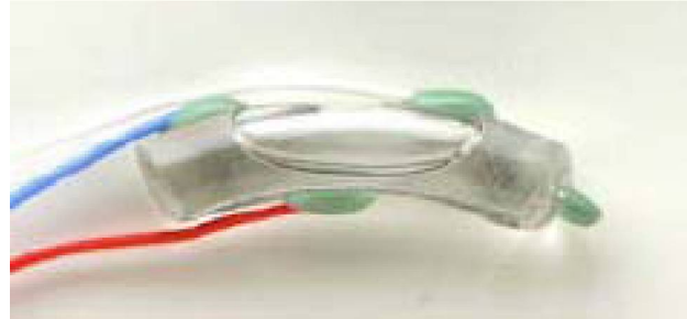
Figure 4.1-8. Electrolytic tilt sensor. This example is from Spectron sensors:
