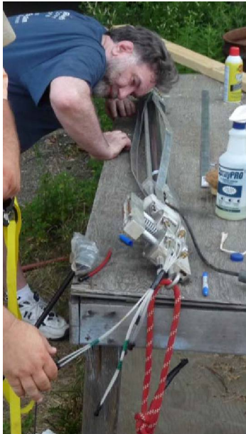
Borehole tiltmeter at NAWC
