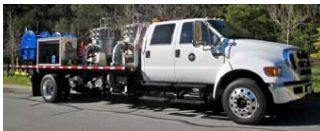
Hillsborough's NO-DES mobile water flushing and filtration unit. Photo courtesy of Hillsborough.
