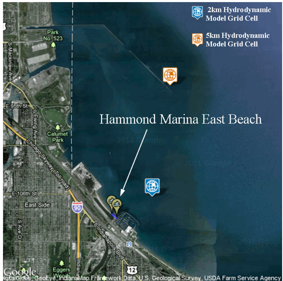
Figure 11.18: Hammond Marina East Beach, Lake County, IN and Hydrodynamic Grid Cell Locations.
