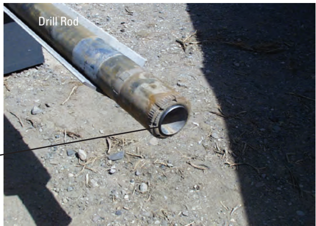
Figure 5. PQ-size coring system similar to one used for coring borehole USGS 136, Idaho National Laboratory, Idaho.
