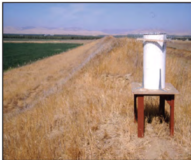
Figure 5. Funnel sampler at the Newman rain gage site at wasteway levee near Draper Road (site 11) in the Central Valley of California. Photograph by Michael Majewski, U.S. Geological Survey.
