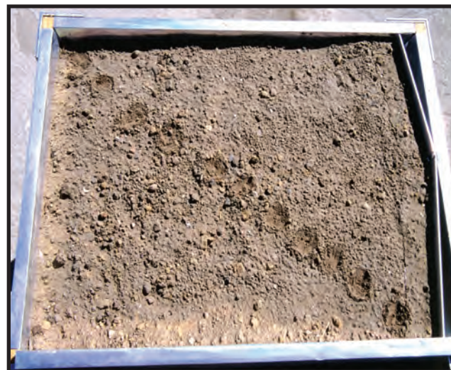
Figure 8. Surficial soil box sampling array. Photograph by Michael Majewski, U.S. Geological Survey.
