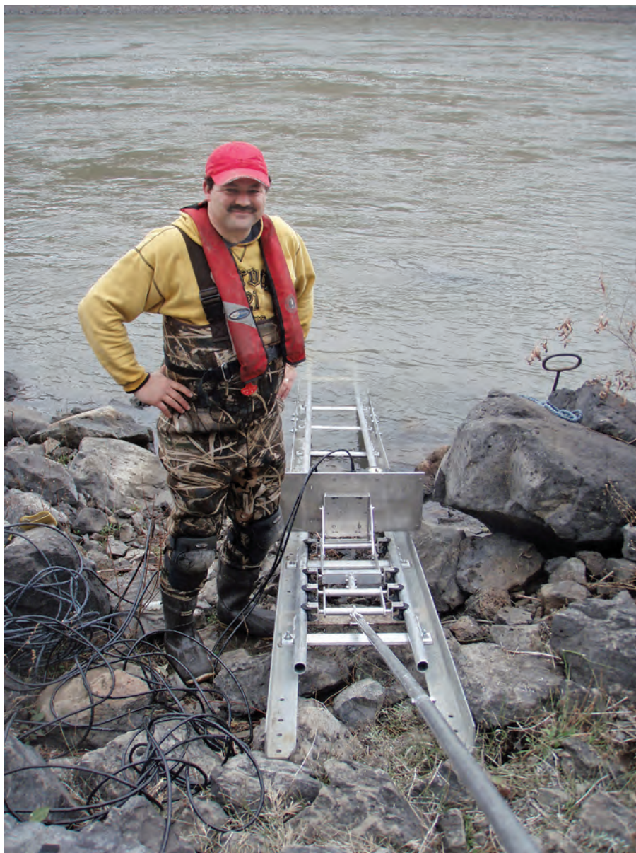
B. The 1.5-MHz and 0.5-MHz SonTek™/YSI acoustic Doppler velocity meters (ADVMS) attached to an aluminum slide track mount about 1,000 ft upstream of the water-quality sonde.
