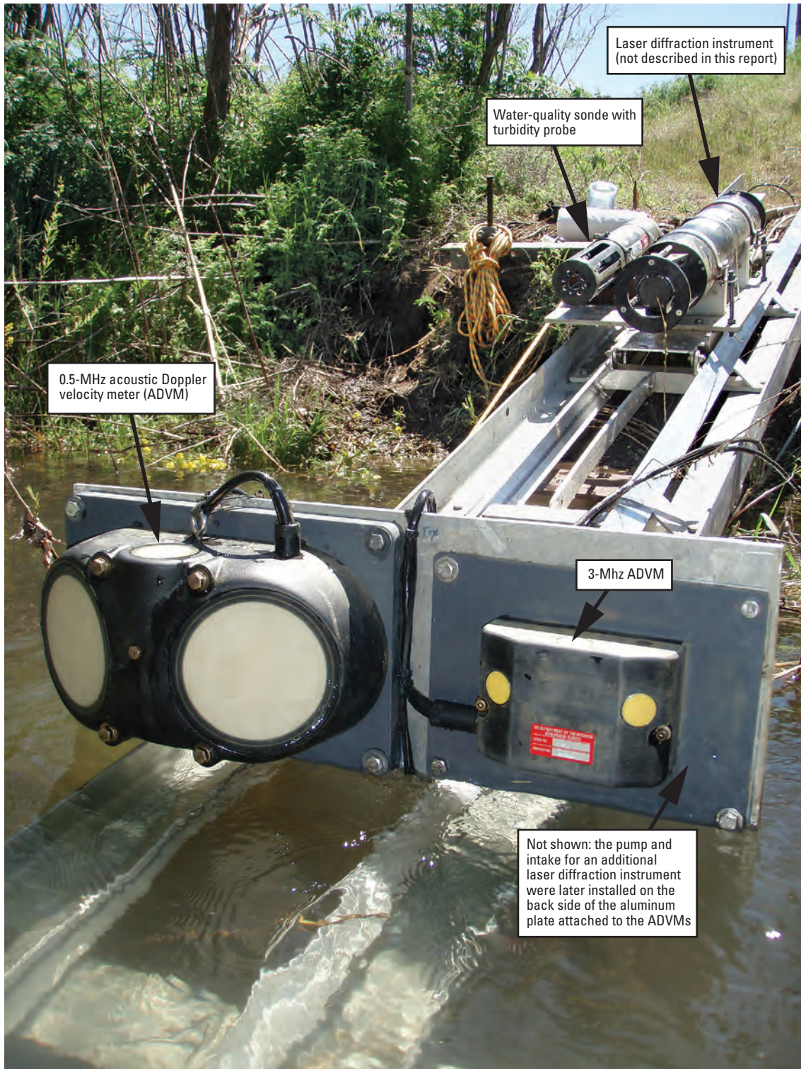
Figure 2. Sediment surrogate instruments deployed at the Clearwater River near Spalding, Idaho. Instruments are shown pulled up the slide track mount for servicing. Not shown: the pump and intake for the LISST-StreamSide was later installed on the back side of the aluminum plate attached to the acoustic Doppler velocity meters. Photograph taken by Molly Wood, U.S. Geological Survey, May 8, 2009.
