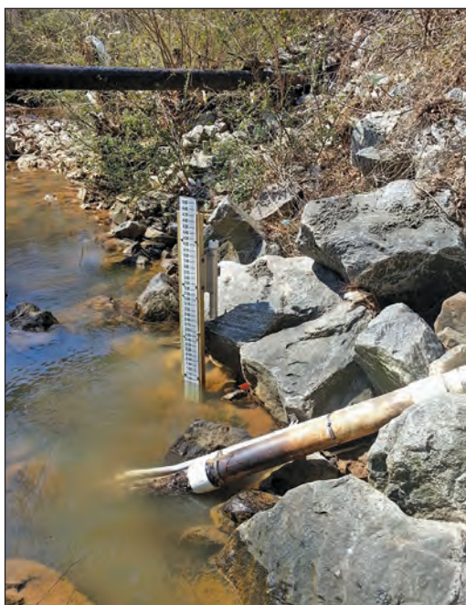
Figure 2. Multiparameter monitoring station at North Fork Peachtree Creek at Graves Road, near Doraville, Georgia. (USGS station number 02336030; photographs by Jonathan Evans, USGS)
