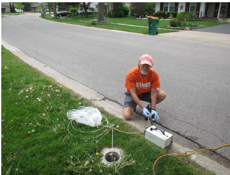
Figure 16. Collection of groundwater samples for analysis of optical brighteners in the study area, Elk Grove Village, Illinois. A , By bailer in observation well TW1. B , By peristaltic pump in well TW9.
