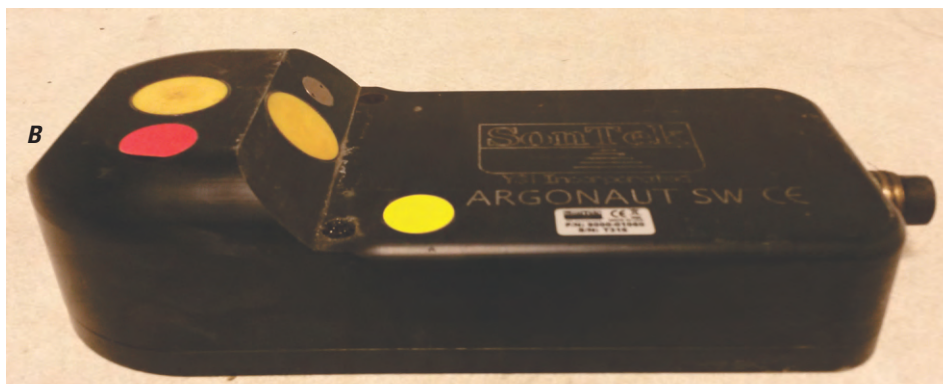
Figure 12. A, Principles of flow measurement with an acoustic Doppler current-velocity meter (ADVM). B, ADVM used in the sanitary sewer installation.
